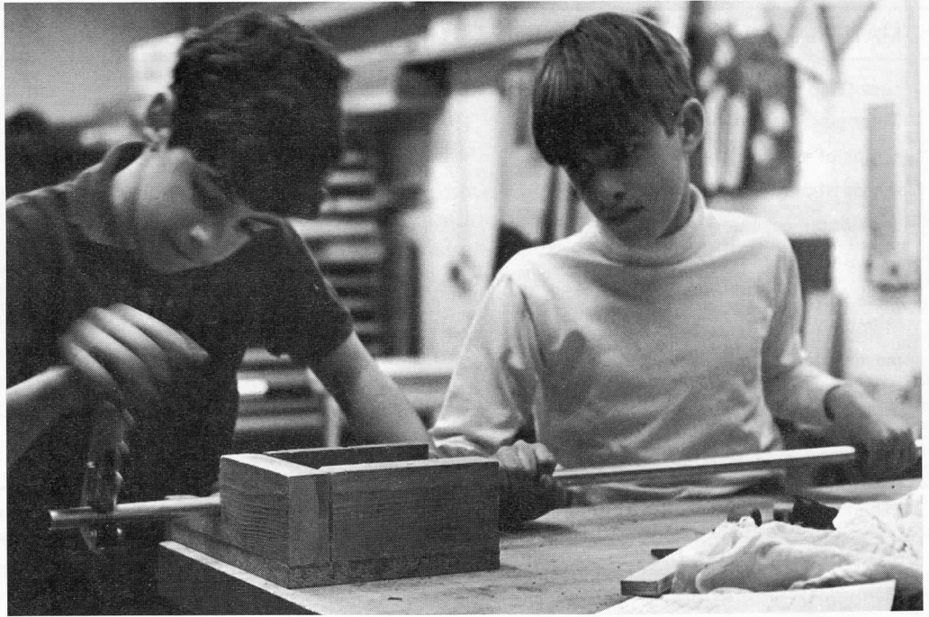
This takes two people—one person to turn the tubing cutter and another to hold the tubing steady.
